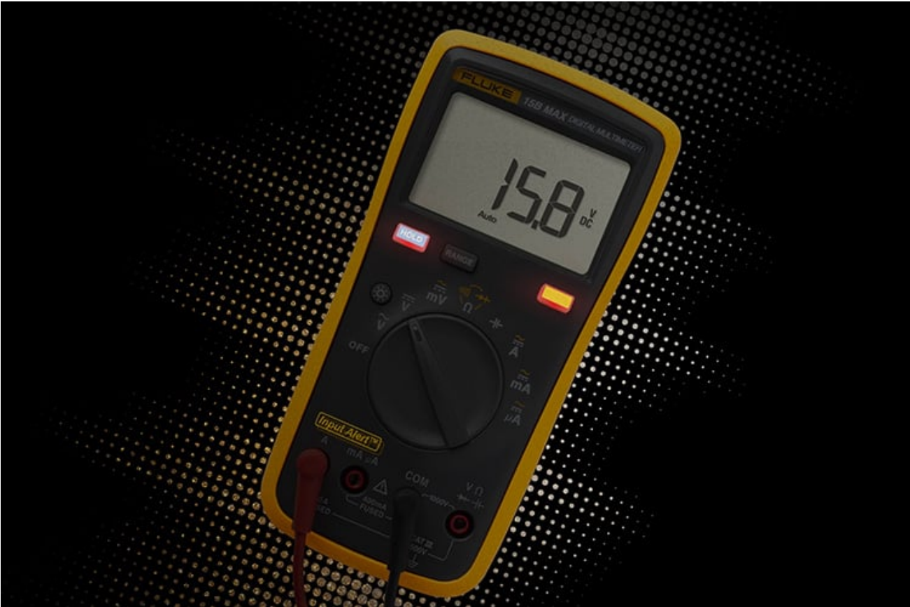
Audible and visual alarm for incorrect connections
